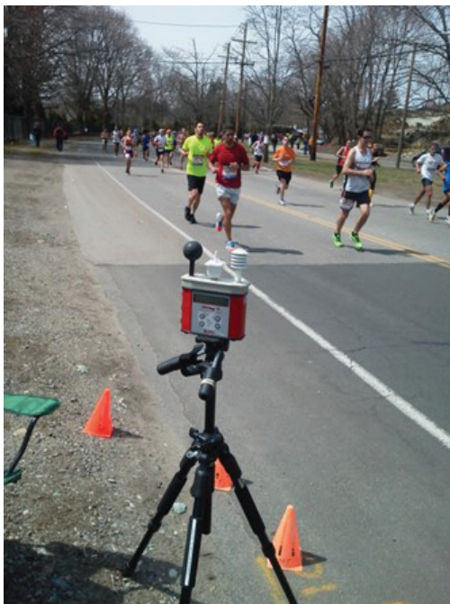
Figure 3. WBGT index measurement made on-site using a sample portable WBGT system. (Runners in Newton, Massachusetts, at the 30 km mark of the 2013 Boston Marathon.)
